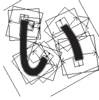
Figure 2. SIFT extracted features from a character image.
