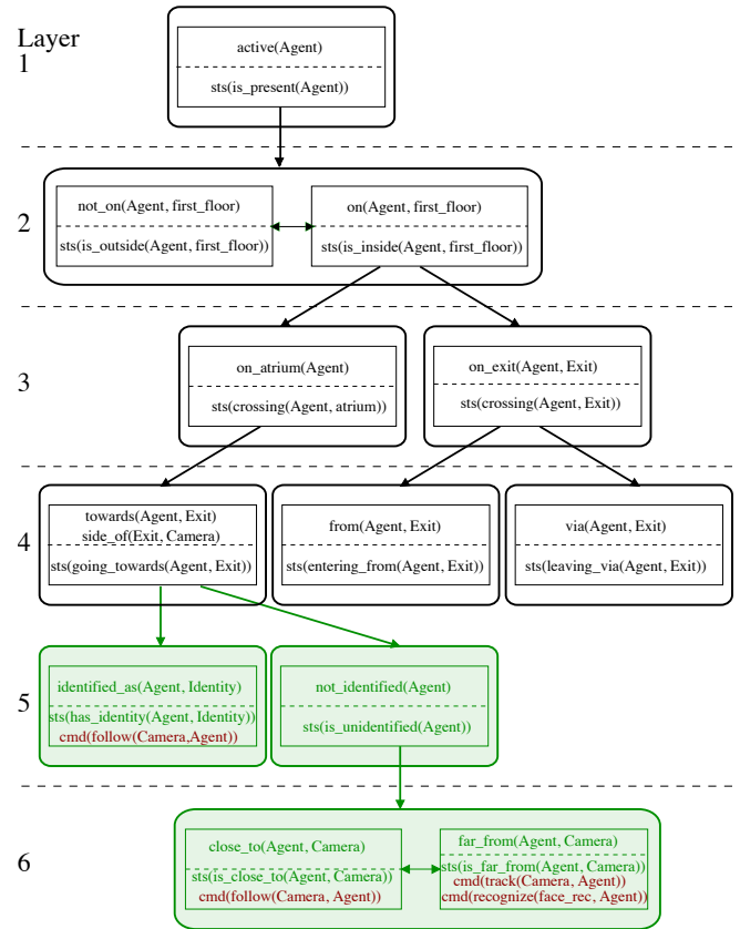
Fig. 4. SGT for active camera selection and face recognition.
