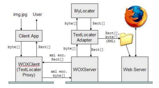
Figure 2. The WOX Client-Server Architecture.
