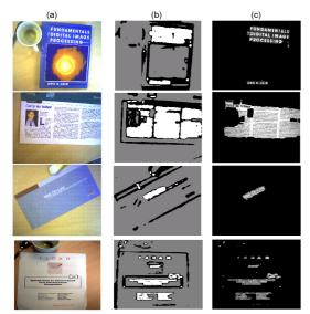
Figure 3. (a) Original images (b) Three-classes clustering (c) Text region
